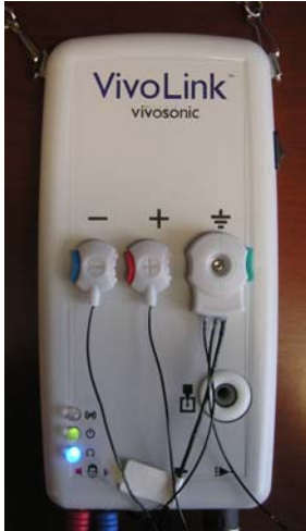
Figure 10. VivoLink™ has no cables connecting it to a computer – it communicates via Bluetooth® wireless communications. The glowing blue LED indicator informs that Bluetooth® is on.
